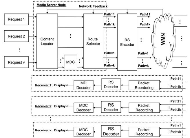
Fig. 2. System Architecture of the proposed error resilient concurrent video streaming over wireless mesh networks using multi-source multi-path transport
