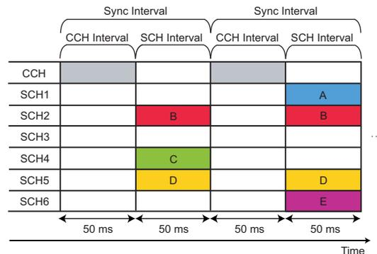
Fig. 1. Schematic diagram of multi-channel operation in IEEE 1609.4 standard.
